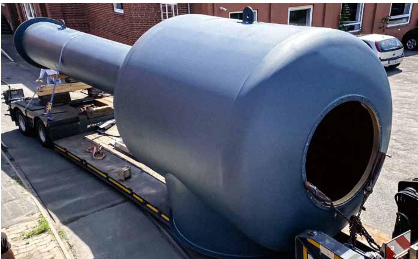
An over 30-metre-long, Körting steam jet compressor at the Hanover site
