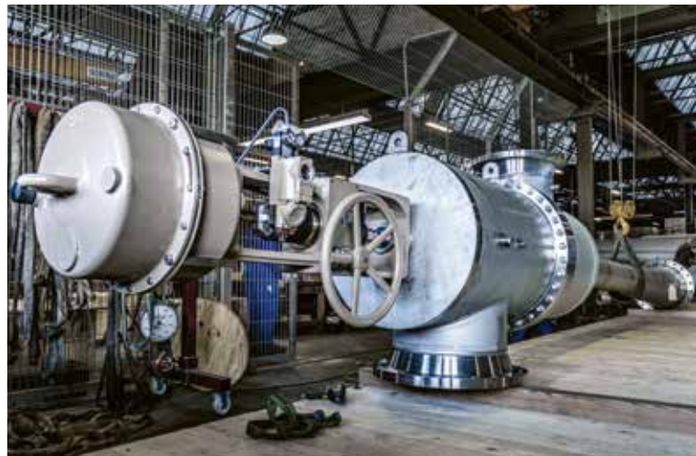
Controllable steam jet compressors with nozzle needle control in the Hanover plant
