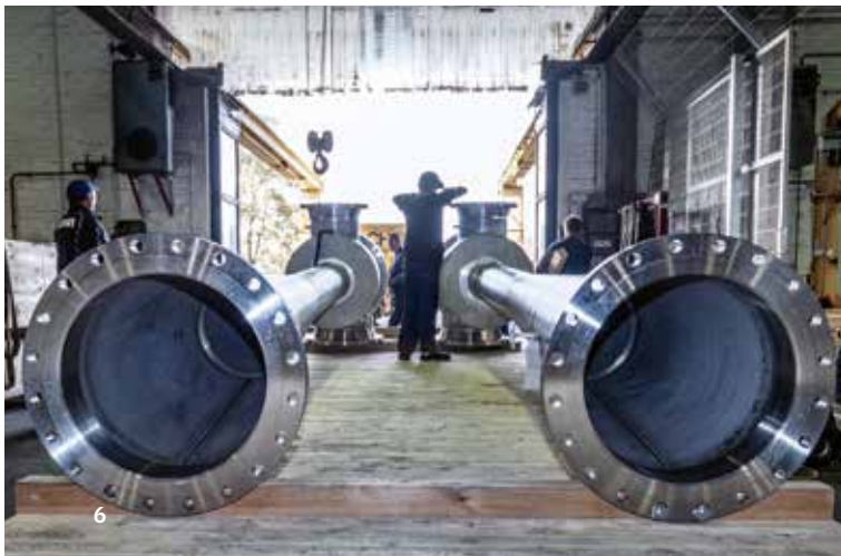
Körting steam jet compressors being loaded
