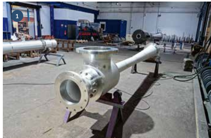
1/2/3) Steam jet compressors being tested
