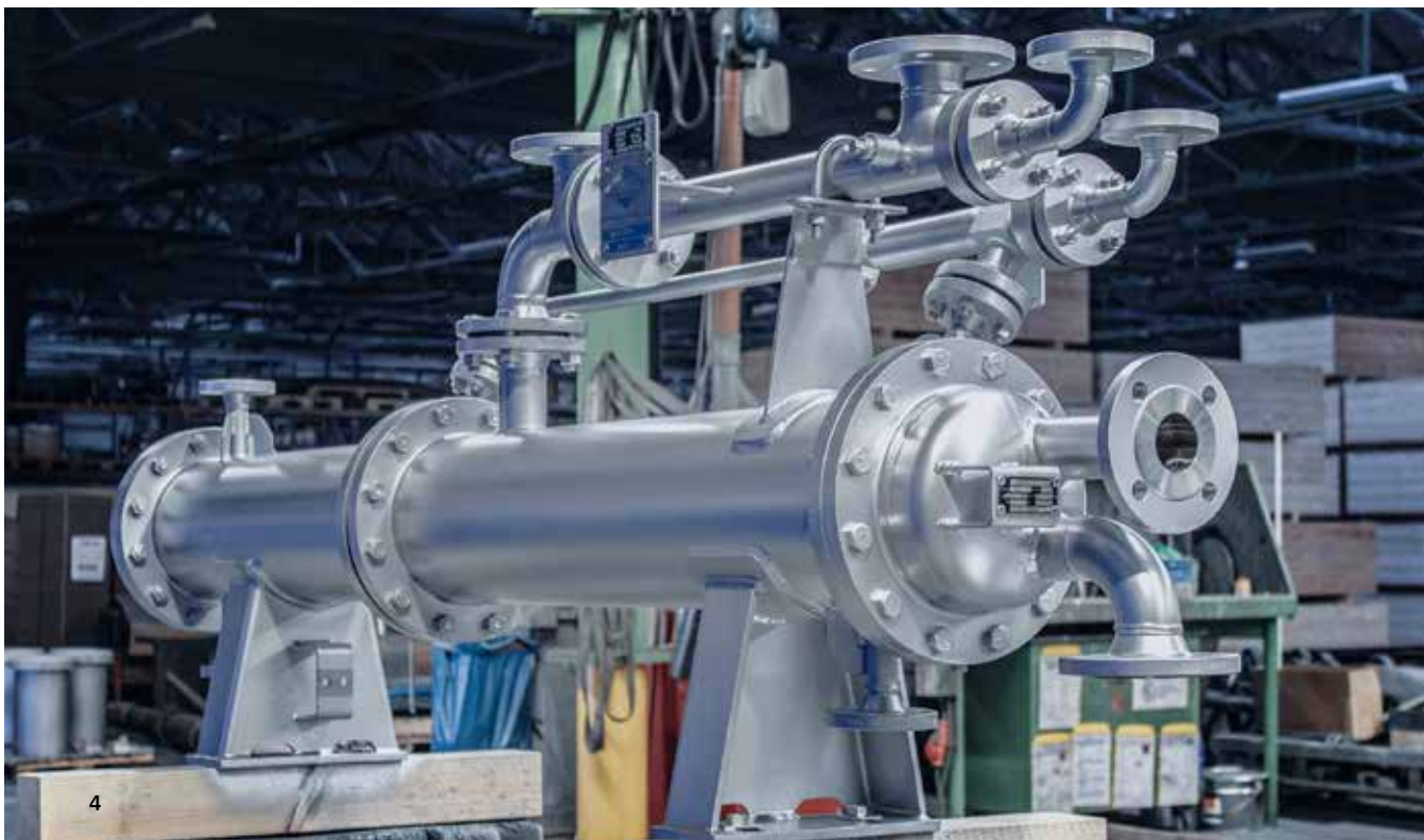
Two-stage, steam jet vacuum system with a surface condenser after final assembly
