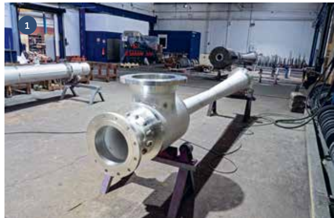
1/2/3) Steam jet compressors being tested
