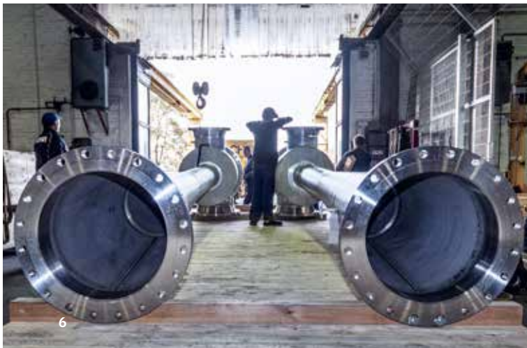
Körting steam jet compressors being loaded
