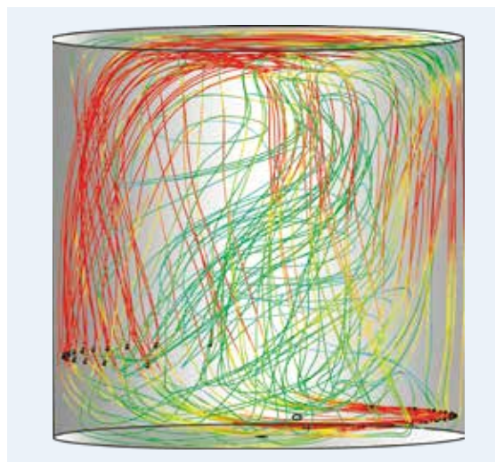
Optimisation of the flow conditions in a cylindrical storage tank for edible oil through three dimensional computer simulation. Vertical section; spatial distribution of the flow velocity as a coloured halftone image
