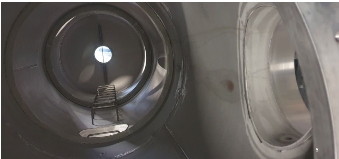
The inside of a vacuum scrubber without fittings
