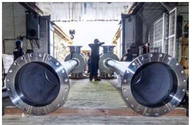
Controllable steam jet compressors with nozzle needle control in the Hanover plant
