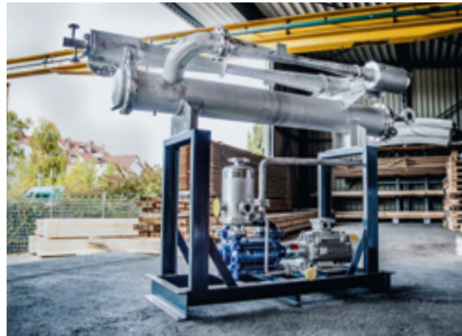
Hybrid system consisting of two steam jet vacuum pumps with surface condenser and a liquid ring vacuum pump
