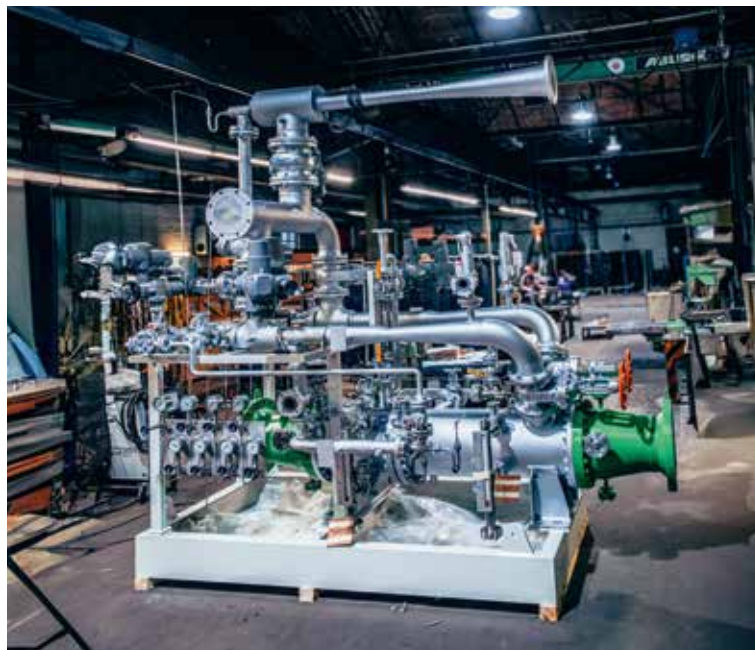
Advanced steam jet vacuum system for removing air from steam turbine condensers with redundant jet ejectors, a double-surface condenser, start-up ejector, silencer, instrumentation, isolation valves and process and motive steam piping
